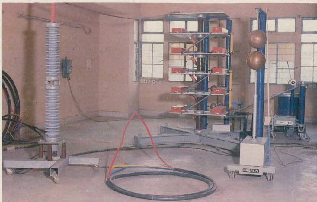
Partial discharge and impulse test for electric cables.
