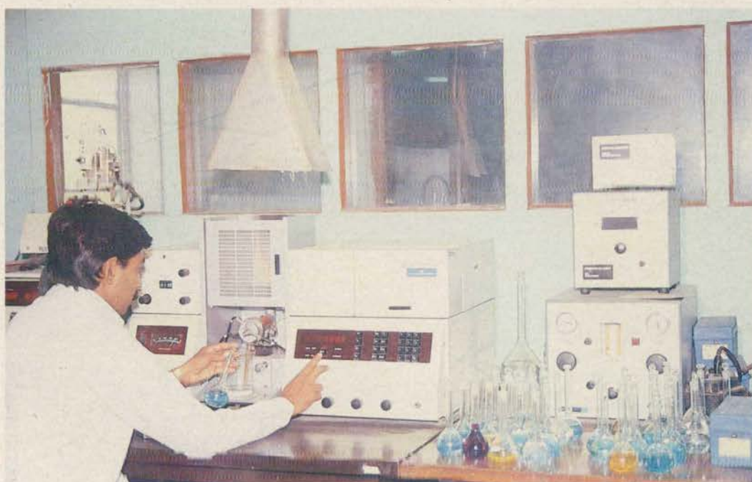
Test of composition of metals by atomic absorption spectrophotometer.
