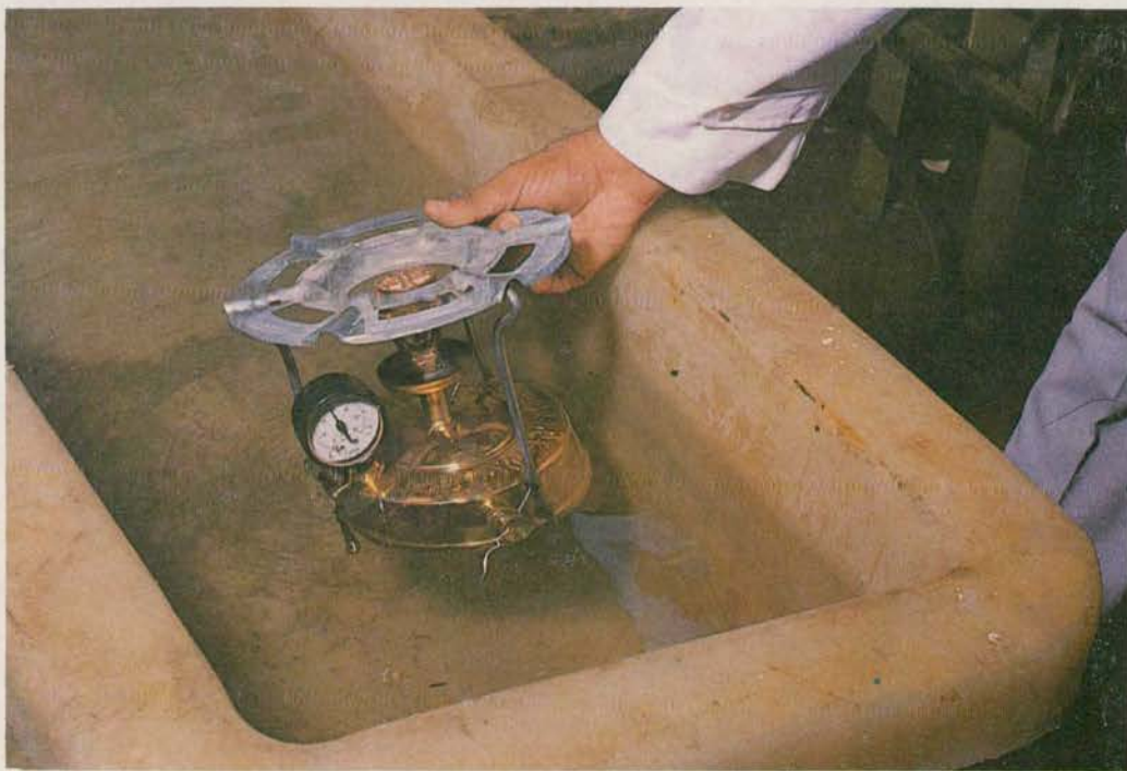
Oil pressure stove being subjected to air pressure test at the Central Laboratory, BIS. To ensure that safe and efficient oil pressure stoves reach the consumers, the Union Ministry of Industry has made the use of the Standard Mark of the Bureau on oil pressure stoves and burners compulsory with effect from 1 October 1987.
