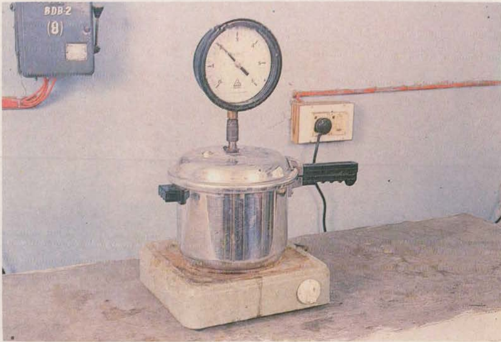
Pressure cooker under test for the operation of safety pressure relief device at the Central Laboratory of the Bureau
